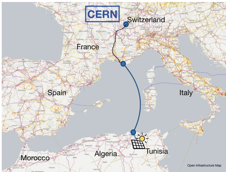
Figure 3.4: Potential CERN-LINK cable (in blue) connecting North African solar power plants with the European electricity grid. Also shown are existing power lines (purple, red, dashed blue), gas and oil pipelines (green/yellow) and photovoltaic (PV) plants (yellow/red dots). Base map taken from Ref. [106], reused and annotated under the terms of the Creative Commons Attribution 4.0 International (CC BY 4.0) license .
