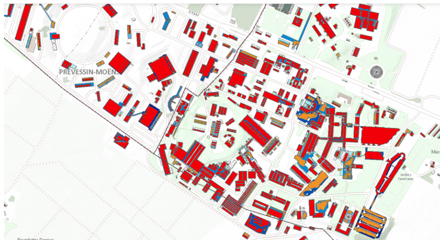
Figure 3.3: Map of CERN buildings. Rooftops that are suitable for PV installation in respect to their received solar irradiation are shown in red (very suitable) and yellow (suitable). In addition other areas like e.g., parking lots could also be covered by PV-panelled roofs. From Ref. [90].
